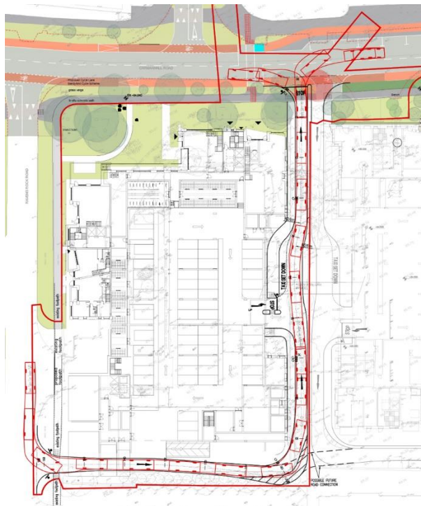
Figure 11 Autotrack Tracking for Fire Tender
