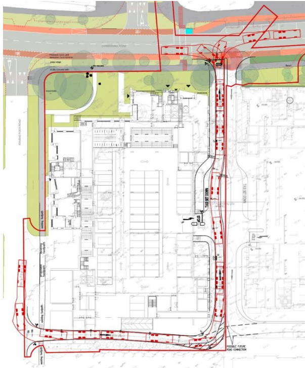
Figure 10 Autotrack Tracking for Refuse Freighter
